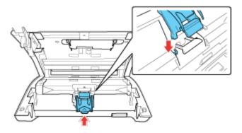
Press the hook on both sides of the paper feed roller cover, then open the cover.
