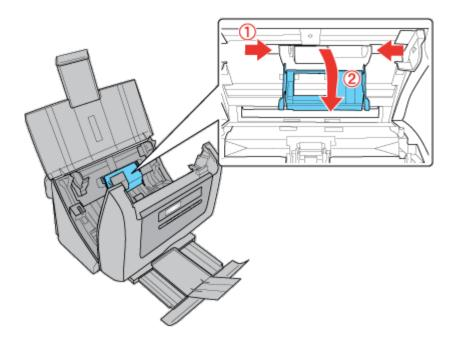
8 Slide and remove the installed paper feed roller.
