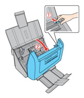
Press the hook on the separation pad, then remove the installed separation pad.
