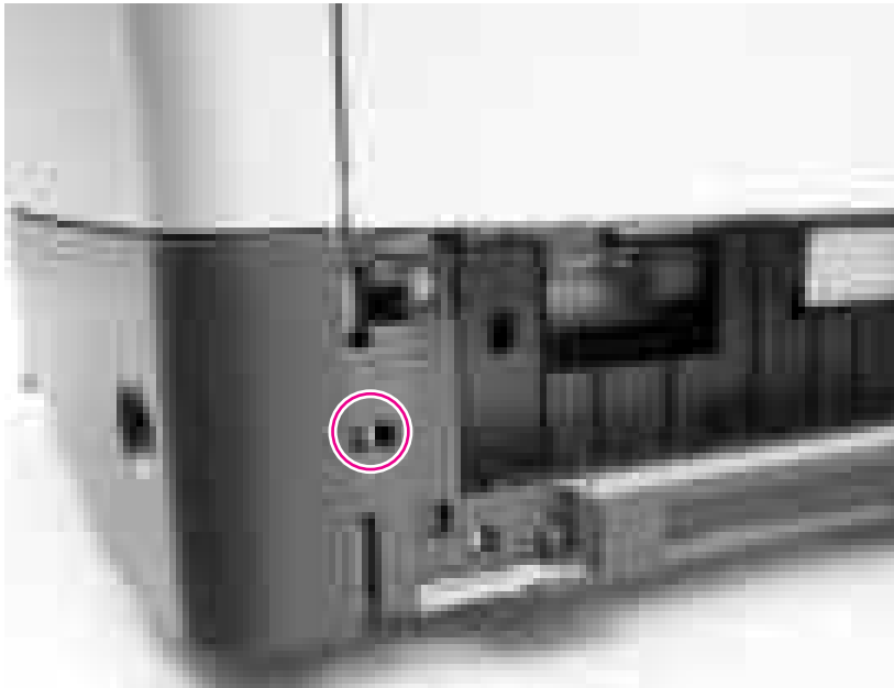
Figure 7-11 Tray 2 jam-access-cover switch, SW105
