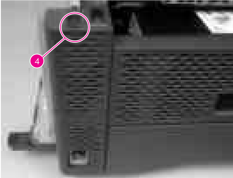
Figure 6-144 Remove the PFC power supply (4 of 8)
