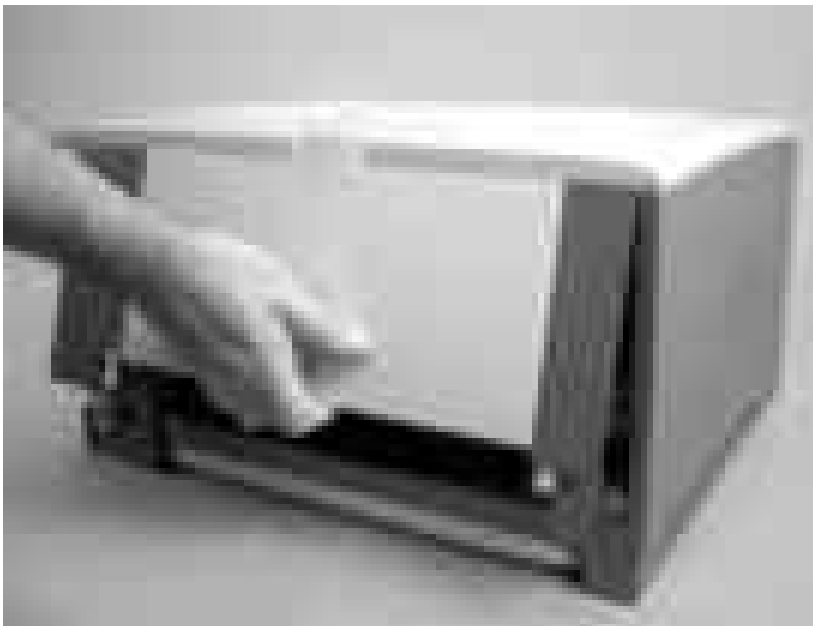
Figure 5-44 Removing the face-up bin (4 of 4)
