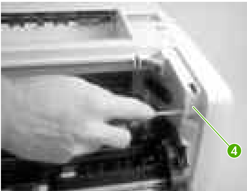
Figure 5-47 Removing the top cover (3 of 5)
