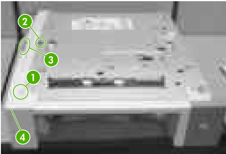
Figure 6-164 Remove the left cover
