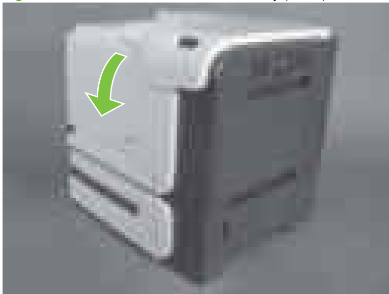
Figure 6-44 Remove the front-door assembly (1 of 2)
