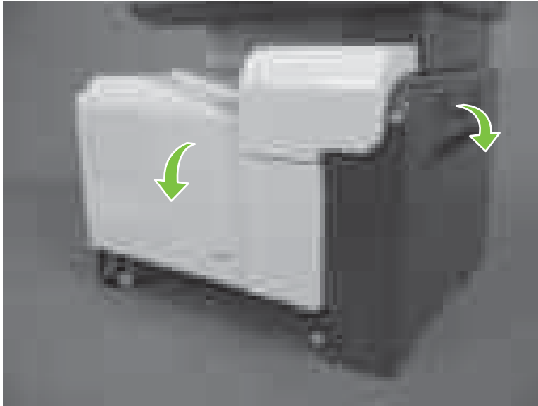
Figure 6-65 Remove the front-upper cover (1 of 4)
