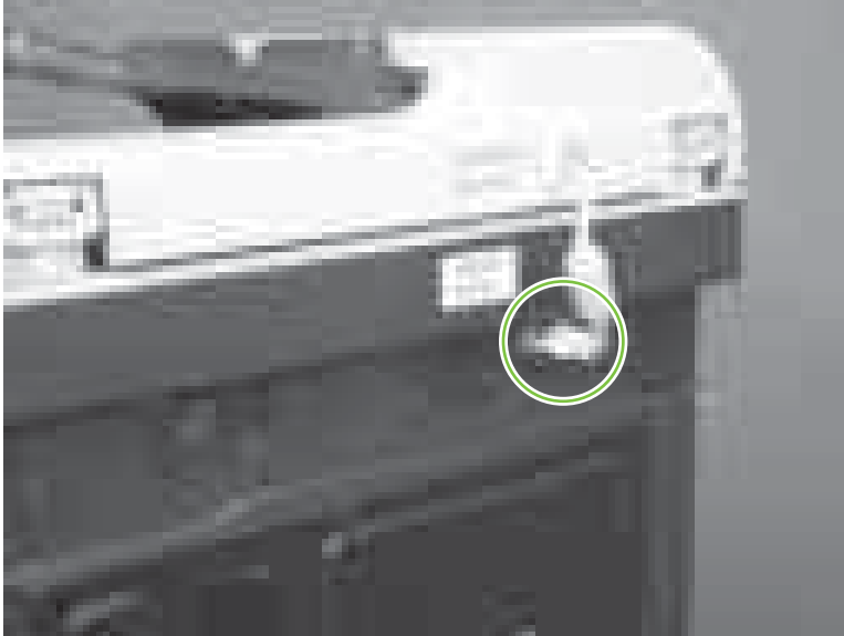
Figure 6-46 Remove the ADF assembly (1 of 4)
