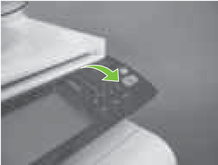
Figure 6-56 Remove the control-panel overlay (1 of 2)
