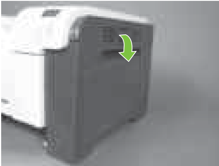
Figure 6-77 Remove the right-rear cover (1 of 3)
