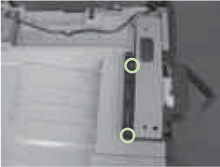
Figure 6-109 Remove the front stapler cover and right-side stapler cover (2 of 13)
