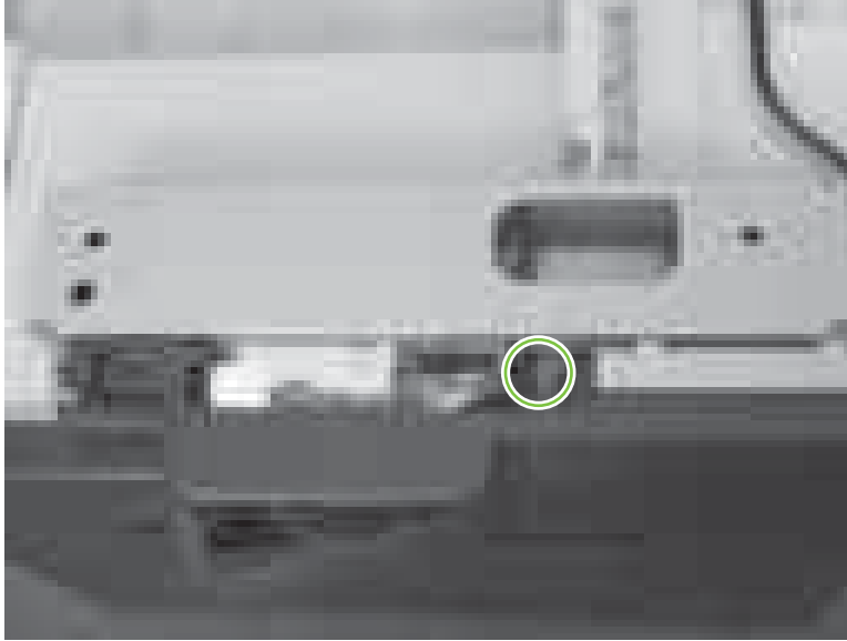
Figure 6-115 Remove the front stapler cover and right-side stapler cover (8 of 13)
