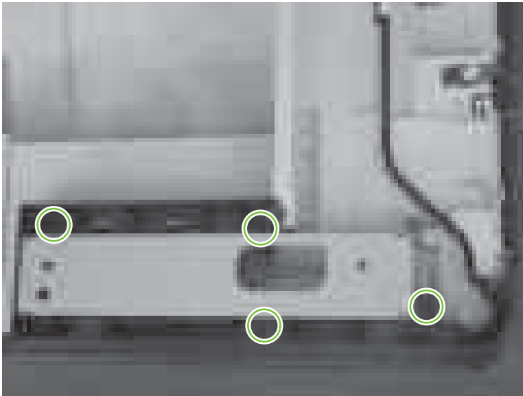
Figure 6-124 Remove the right-top cover (1 of 5)
