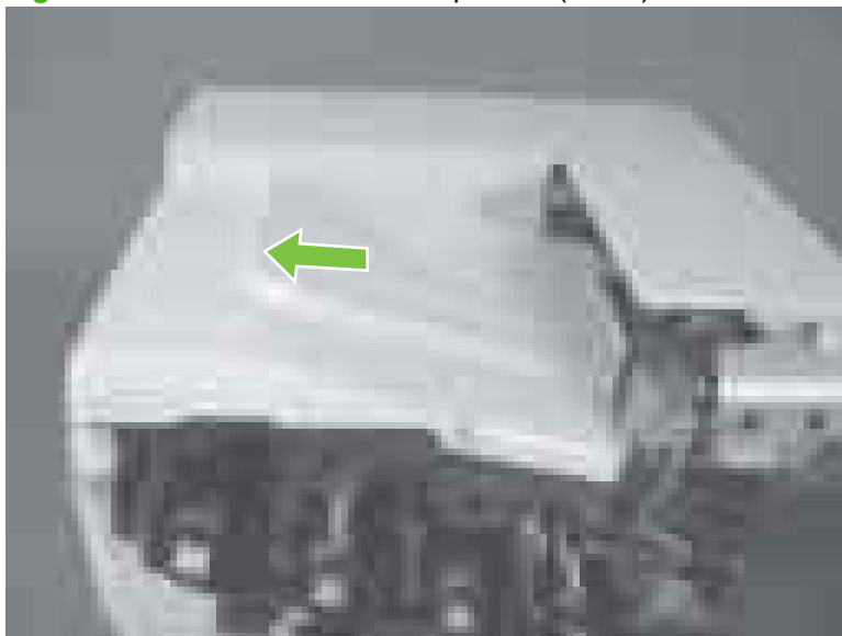
Figure 6-130 Remove the front-top cover (2 of 2)
