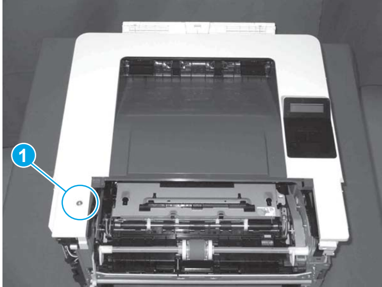
Figure 1-1221 Remove one screw
