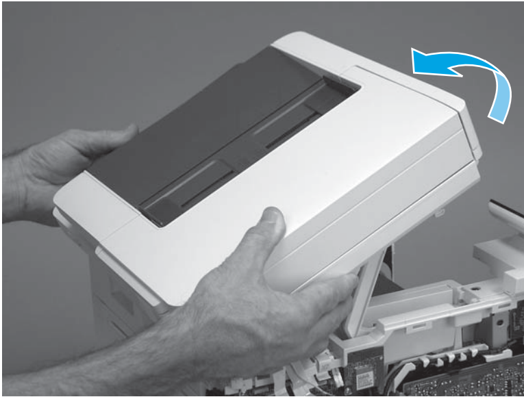
Figure 1-1365 Rotate the ISA towards the rear of the printer
