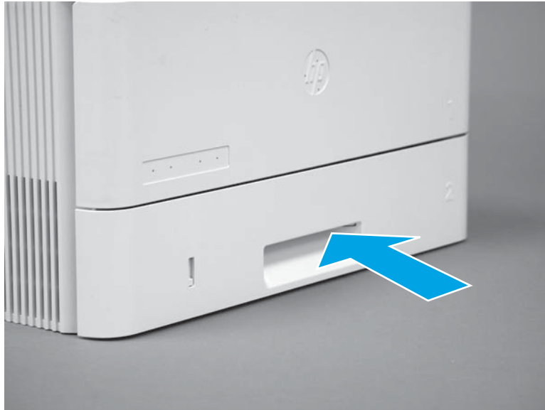
Figure 1-1543 Install the tray
