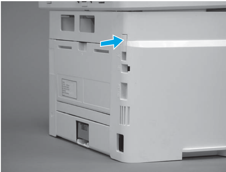
Figure 1-63 Install the cover
