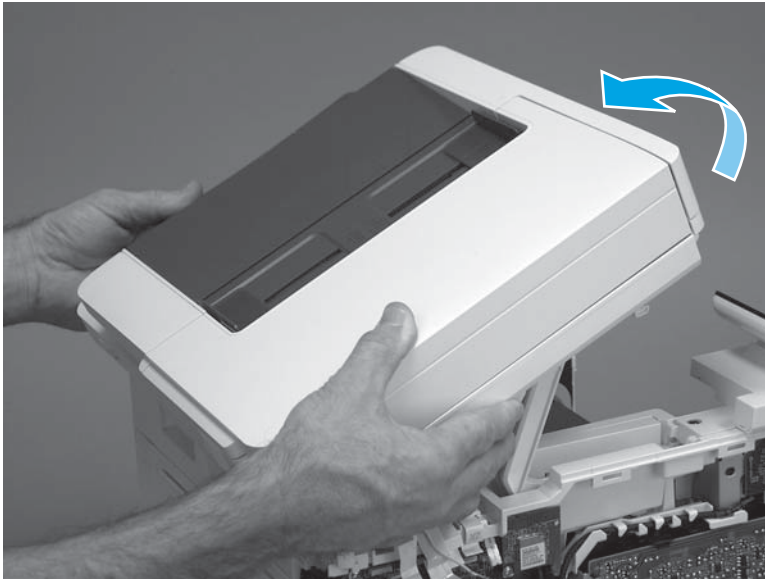
Figure 1-1048 Rotate the ISA towards the rear of the printer
