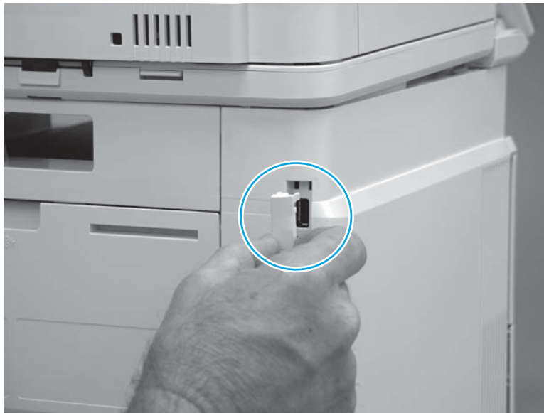
Figure 1-98 Remove the cover
