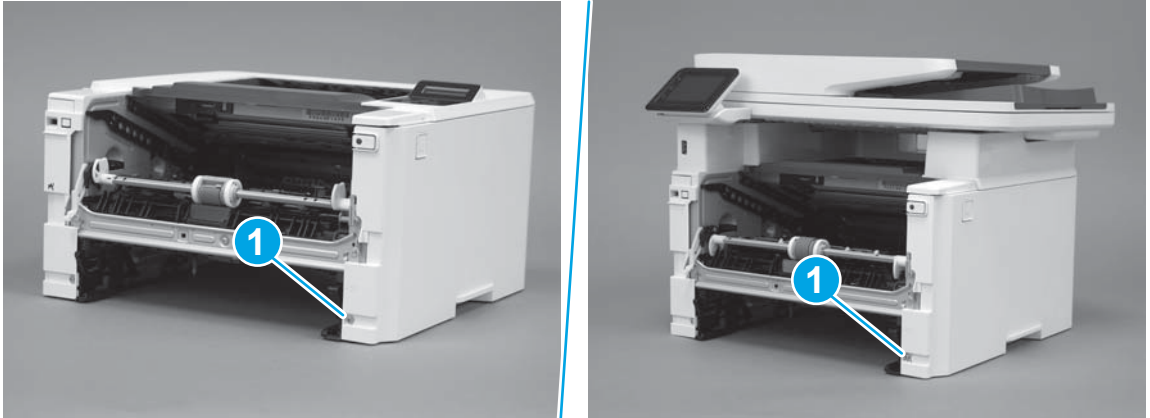
Figure 1-714 Install one screw
