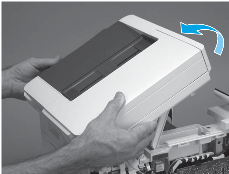
Figure 1-1980 Rotate the ISA towards the rear of the printer
