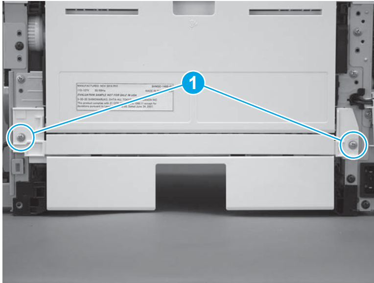
Figure 1-160 Install two screws
