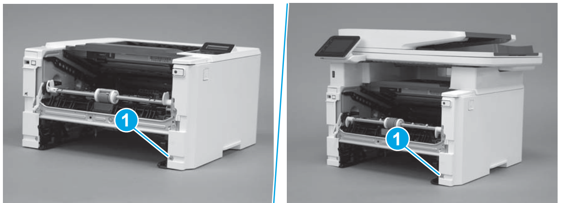
Figure 1-136 Install one screw
