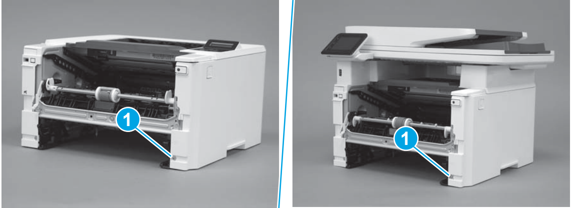
Figure 1-296 Remove one screw
