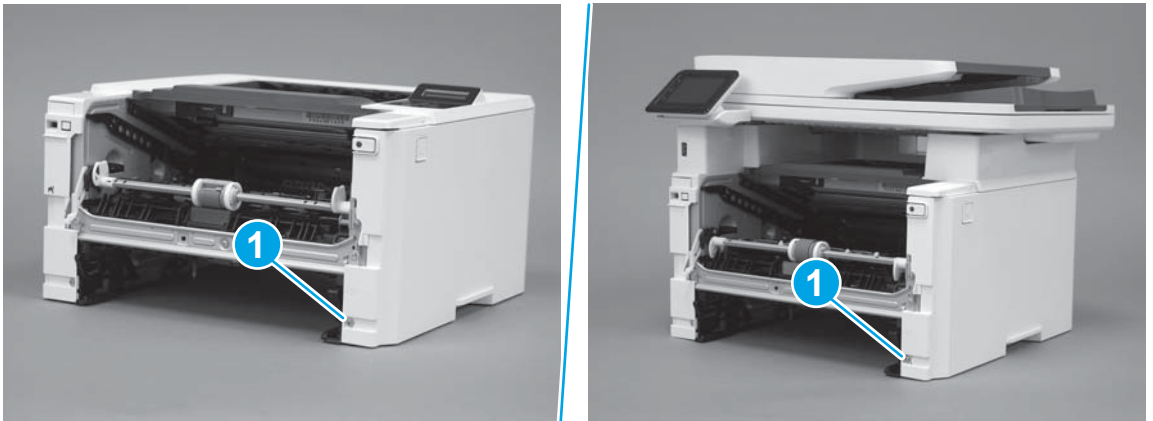
Figure 1-1353 Remove one screw
