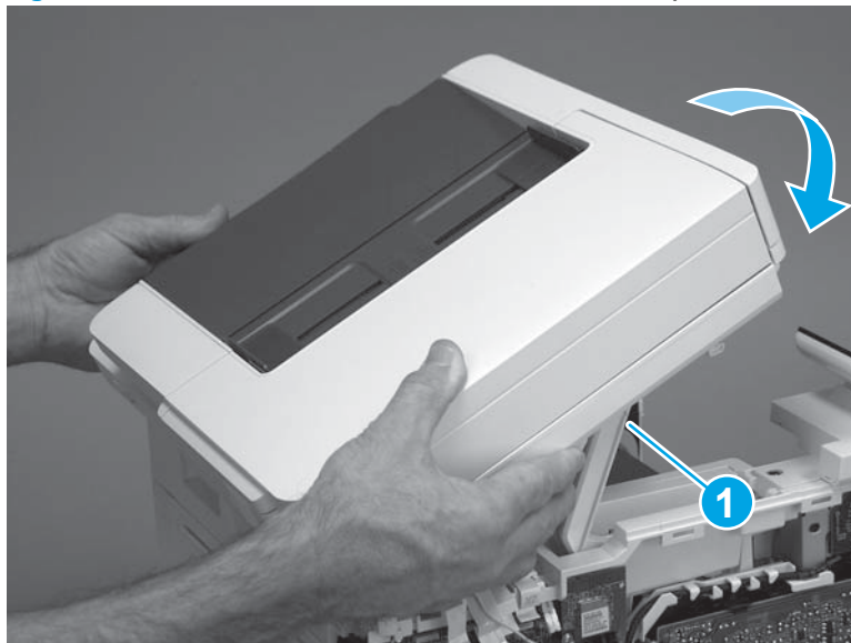
Figure 1-1322 Rotate the ISA towards the front of the printer
