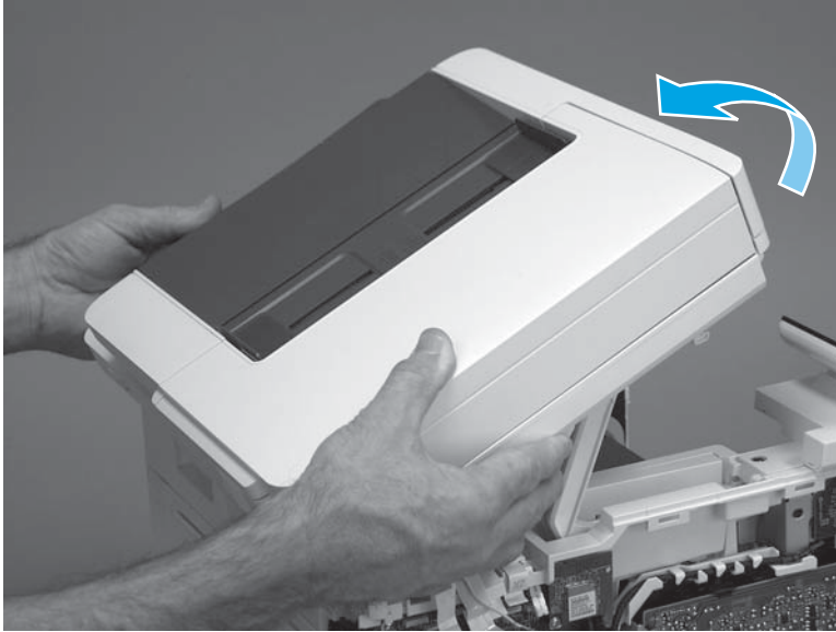
Figure 1-639 Rotate the ISA towards the rear of the printer
