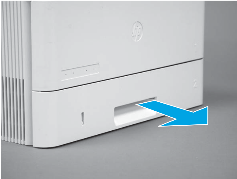
Figure 1-888 Remove the tray
