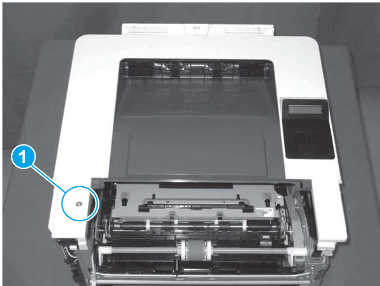
Figure 1-652 Remove one screw
