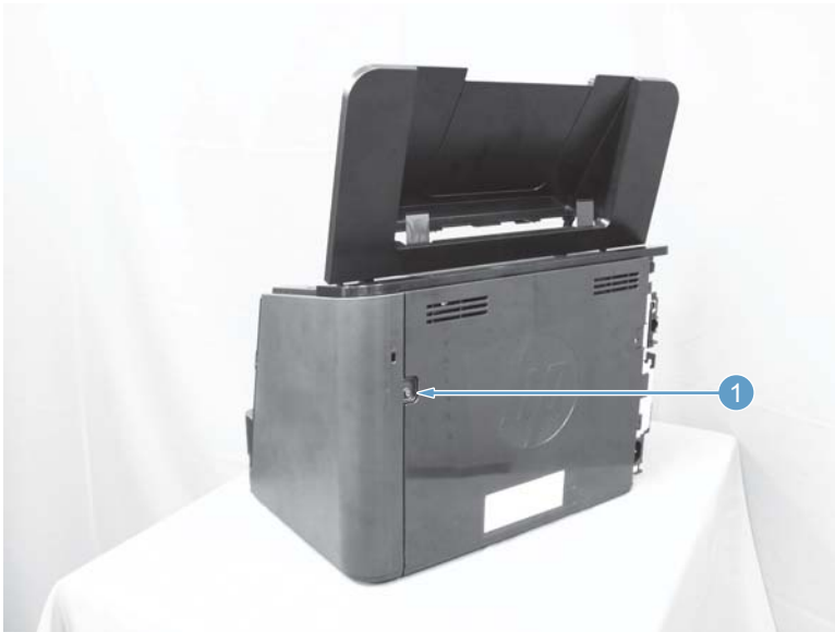
Figure 1-21 Remove the right cover, simplex product (1 of 2)
