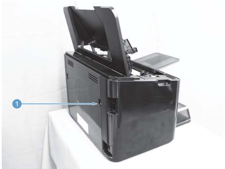
Figure 1-13 Remove the left cover, simplex product (1 of 2)
