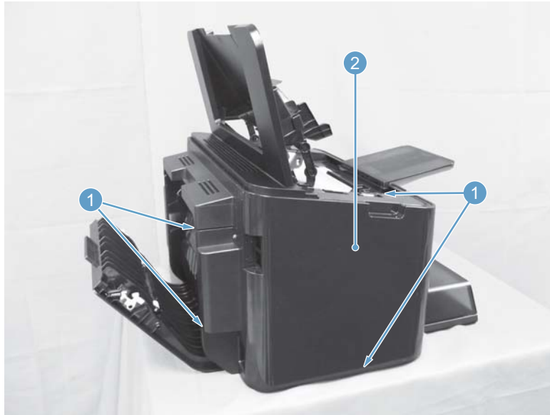
Figure 1-12 Remove the left cover, duplex product (2 of 2)
