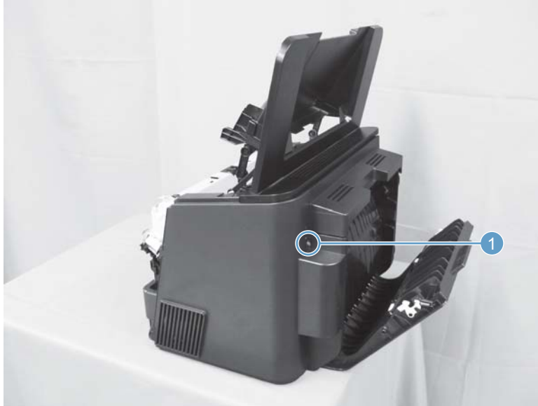
Figure 1-19 Remove the right cover, duplex product (1 of 2)
