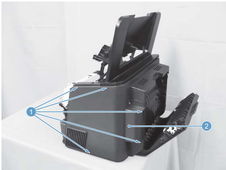
Figure 1-20 Remove the right cover, duplex product (2 of 2)
