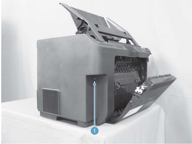
Figure 1-53 Remove the right cover (1 of 3)
