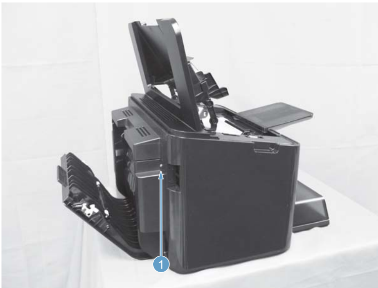
Figure 1-11 Remove the left cover, duplex product (1 of 2)
