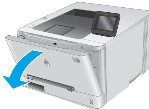
Figure 1-557 Open the front door and rear door or duplexer door (1 of 2)
