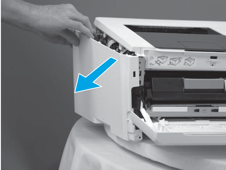
Figure 1-184 Remove the left cover (3 of 3)
