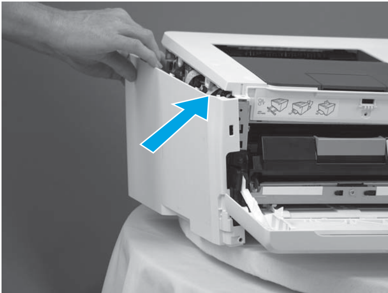
Figure 1-291 Install the left cover (1 of 3)
