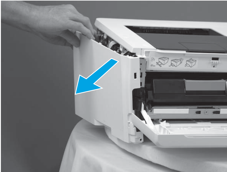
Figure 1-370 Remove the left cover (3 of 3)
