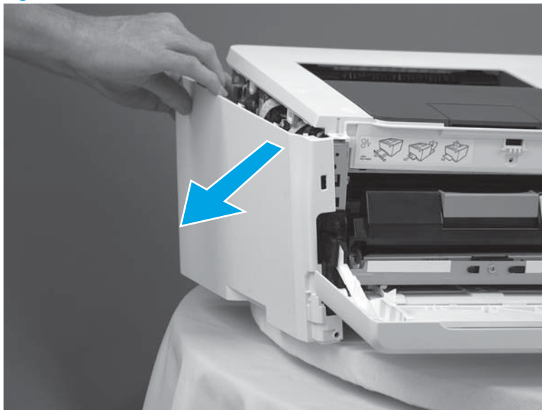
Figure 1-649 Remove the left cover (3 of 3)
