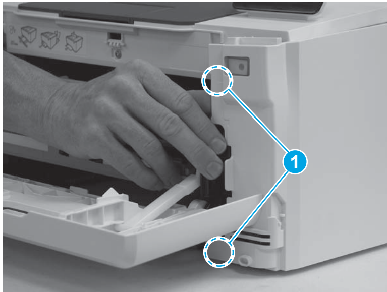
Figure 1-744 Install the right cover (1 of 3)
