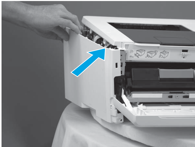
Figure 1-49 Install the left cover (1 of 3)
