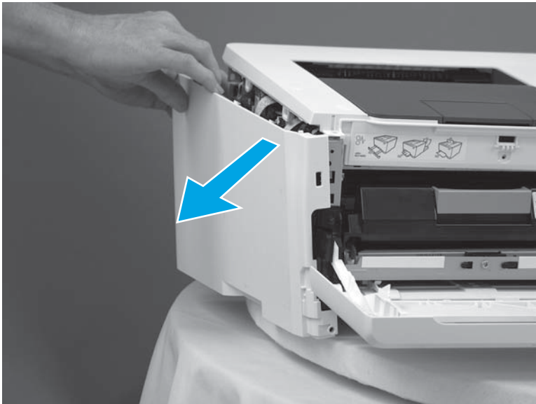
Figure 1-287 Remove the left cover (3 of 3)
