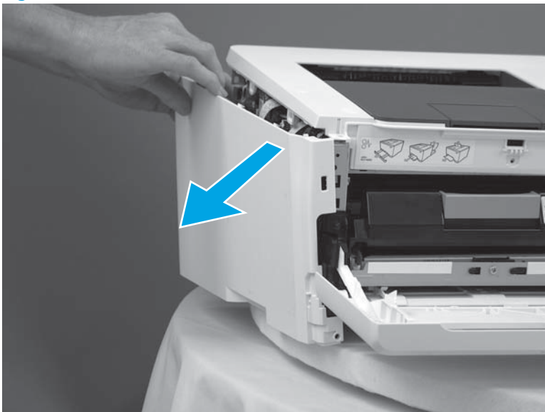
Figure 1-47 Remove the left cover (3 of 3)
