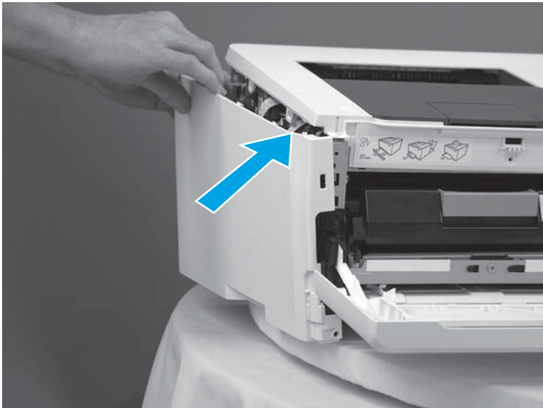
Figure 1-325 Install the left cover (1 of 3)
