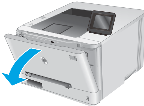
Figure 1-392 Open the front door and rear door or duplexer door (1 of 2)
