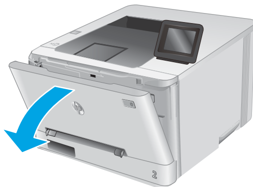
Figure 1-751 Open the front door and rear door or duplexer door (1 of 2)
