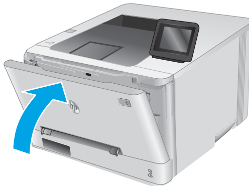
Figure 1-421 Close the front door and rear door or duplexer door (1 of 2)
