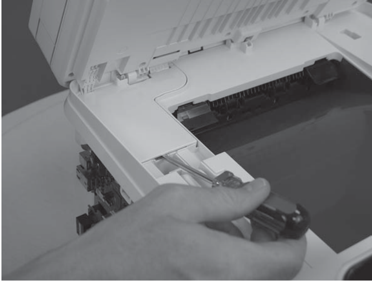
Figure 1-241 Remove the M274, M277 scanner (2 of 4)
