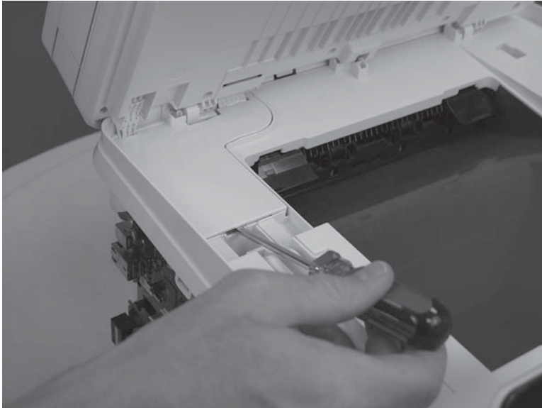
Figure 1-651 Remove the M274, M277 scanner (2 of 4)
