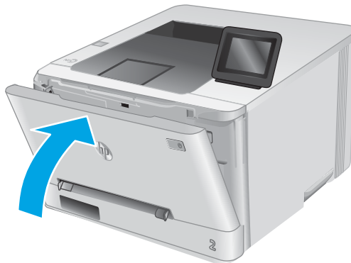
Figure 1-452 Close the front door and rear door or duplexer door (1 of 2)
