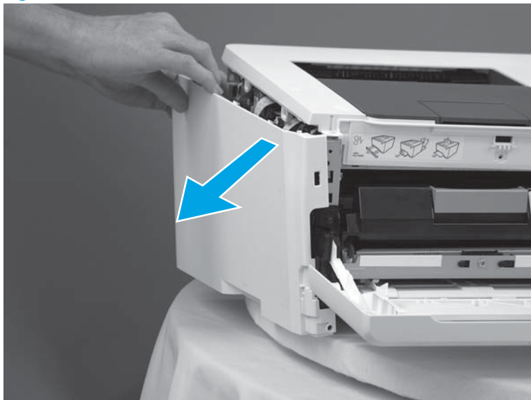
Figure 1-272 Remove the left cover (3 of 3)
