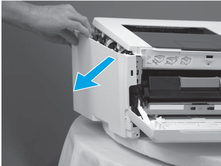
Figure 1-116 Remove the left cover (3 of 3)
