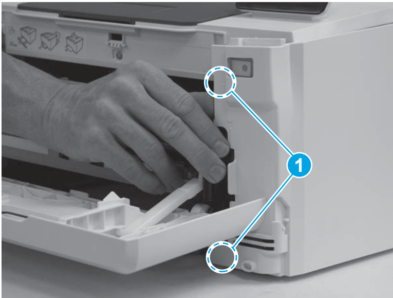
Figure 1-618 Install the right cover (1 of 3)
