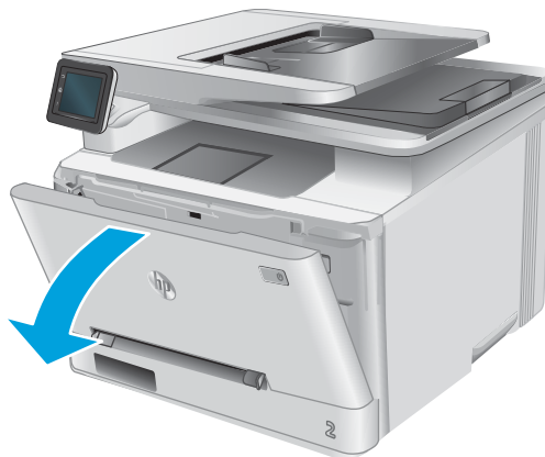
Figure 1-298 Open the front door and rear door or duplexer door (1 of 2)
