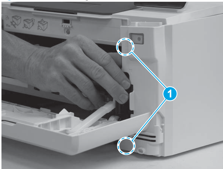
Figure 1-550 Install the right cover (1 of 3)
