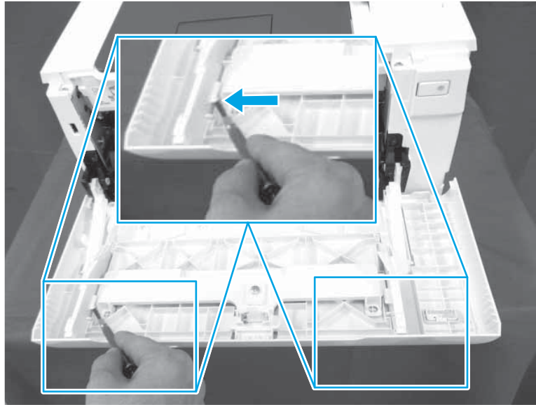
Figure 1-220 Remove the front door (2 of 2)
