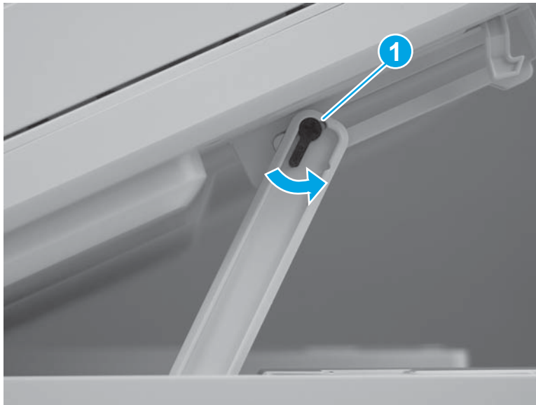
Figure 1-117 Remove the M274, M277 scanner (1 of 4)
