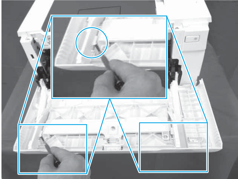
Figure 1-222 Install the front door
