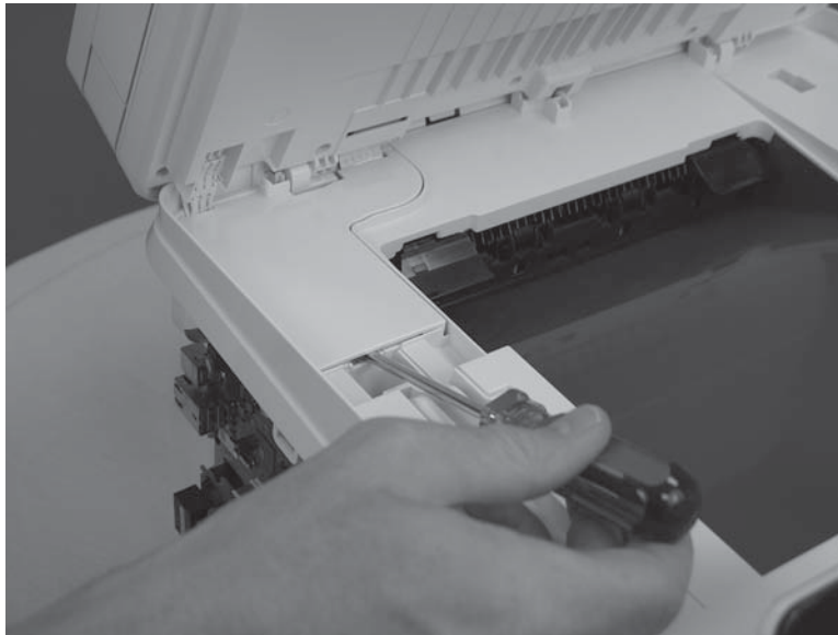
Figure 1-709 Install the M274, M277 scanner (3 of 4)
