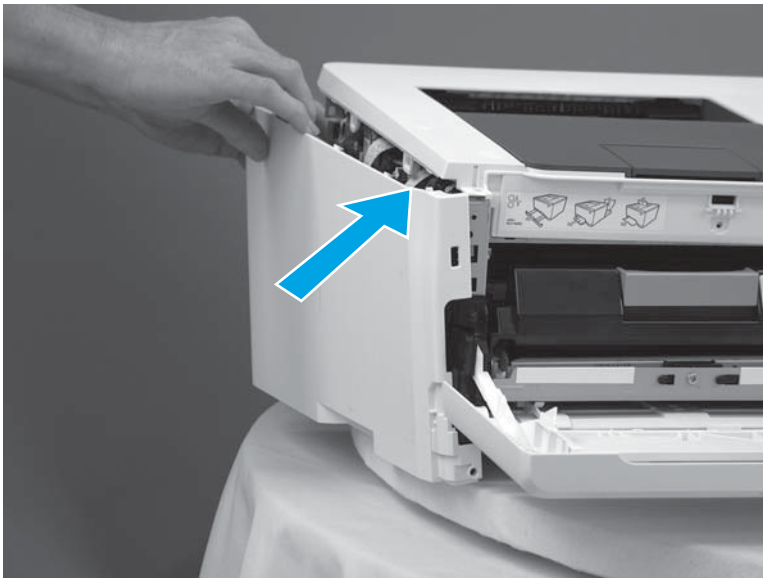
Figure 1-711 Install the left cover (1 of 3)
