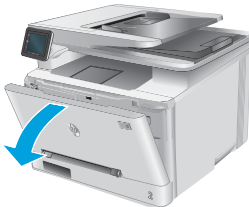
Figure 1-232 Open the front door and rear door or duplexer door (1 of 2)
