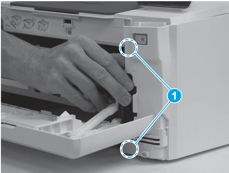
Figure 1-635 Install the right cover (1 of 3)
