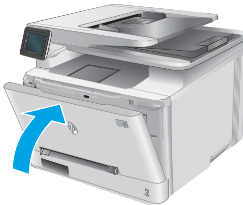
Figure 1-387 Close the front door and rear door or duplexer door (1 of 2)
