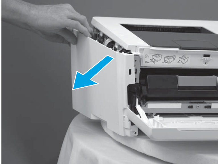
Figure 1-239 Remove the left cover (3 of 3)
