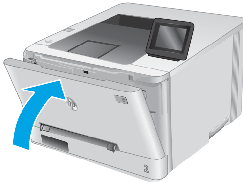
Figure 1-553 Close the front door and rear door or duplexer door (1 of 2)
