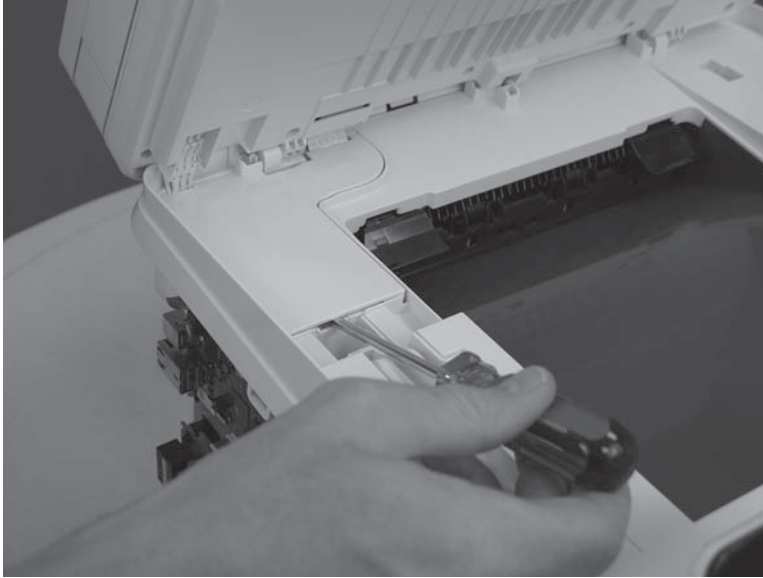
Figure 1-247 Install the M274, M277 scanner (3 of 4)
