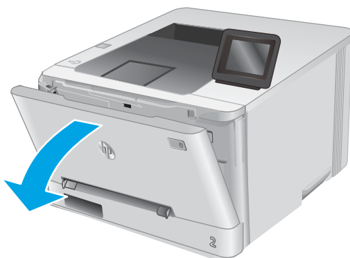
Figure 1-736 Open the front door and rear door or duplexer door (1 of 2)
