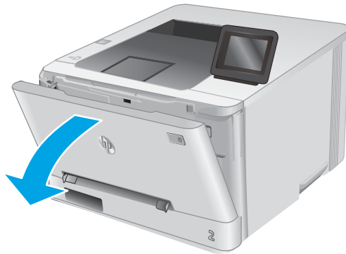
Figure 1-427 Open the front door and rear door or duplexer door (1 of 2)
