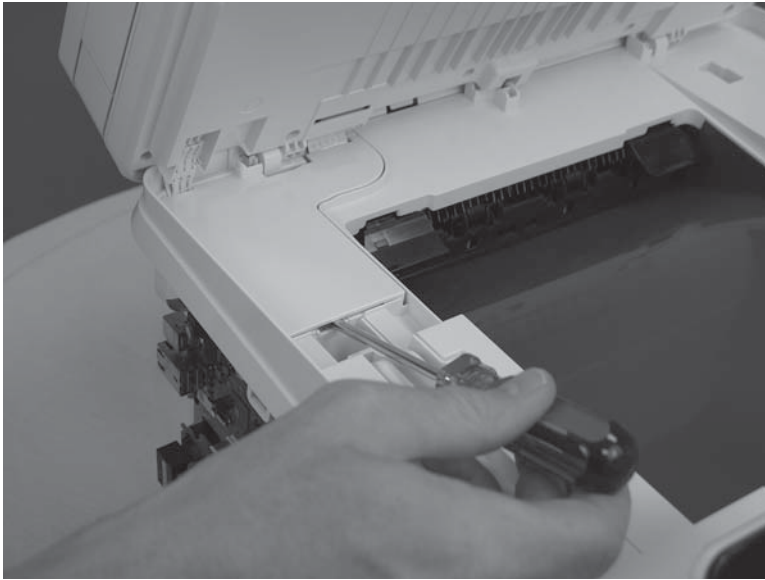
Figure 1-118 Remove the M274, M277 scanner (2 of 4)
