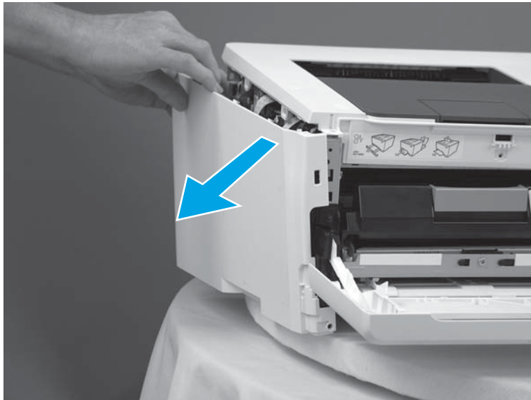
Figure 1-302 Remove the left cover (3 of 3)
