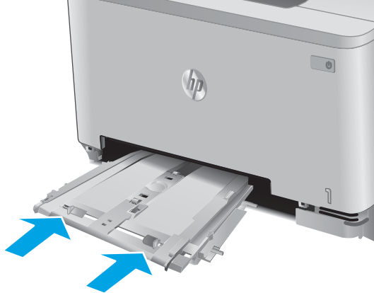
Figure 1-5 Install the priority feed slot tray
