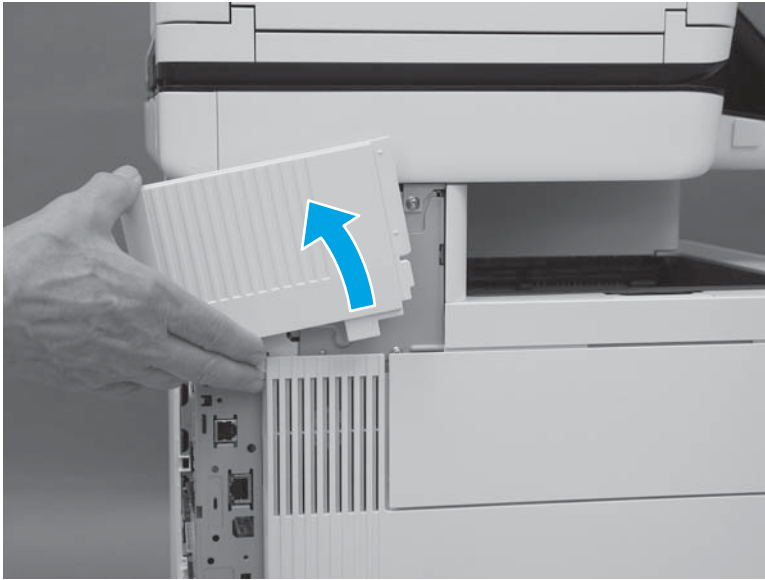
Figure 1-4332 Remove the left upper cover
