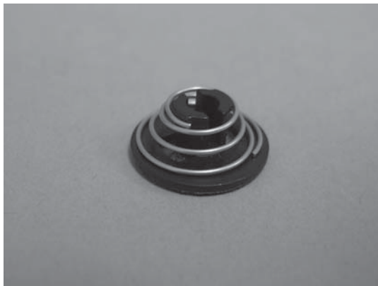
Figure 1-165 Check the retention clip spring
