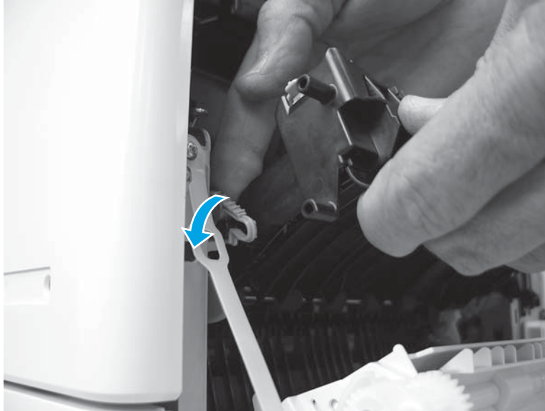
Figure 1-4020 Carefully flex the top portion of the blue arm
