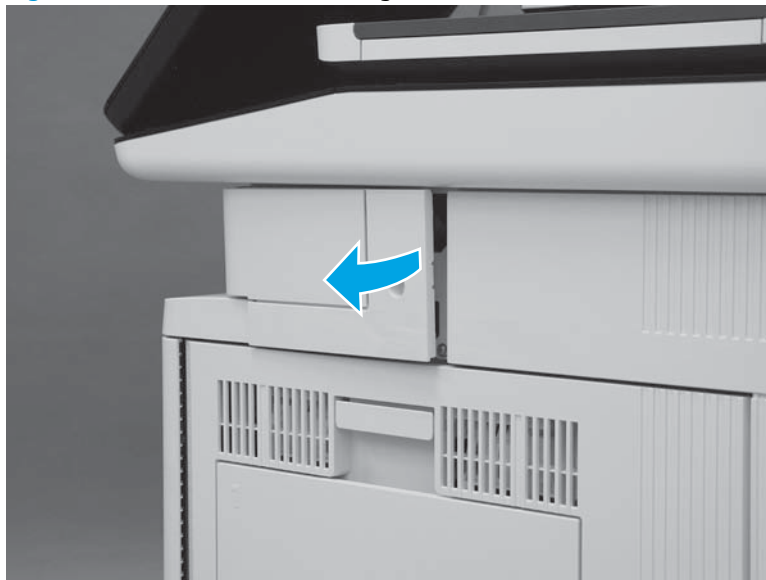
Figure 1-330 Release the back edge of the cover
