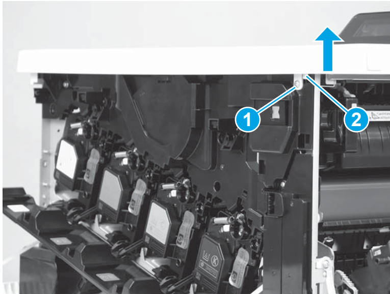
Figure 1-3026 Remove one screw and release one tab
