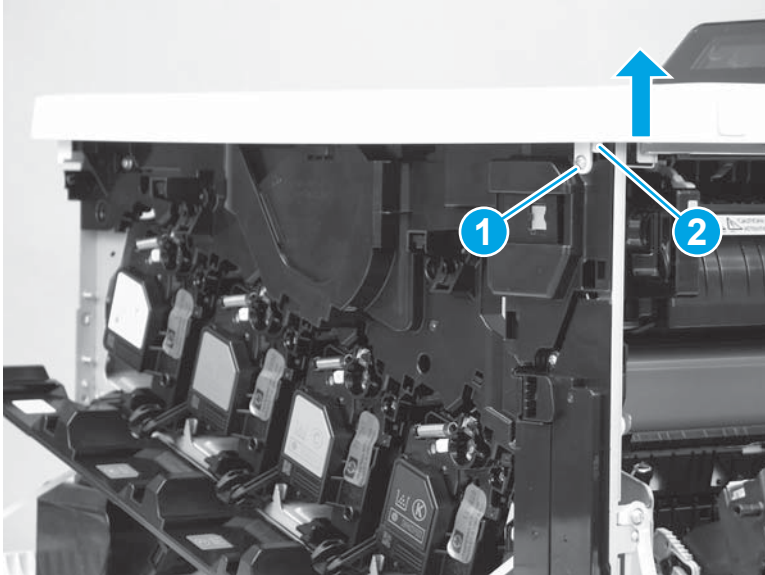
Figure 1-681 Remove one screw and release one tab
