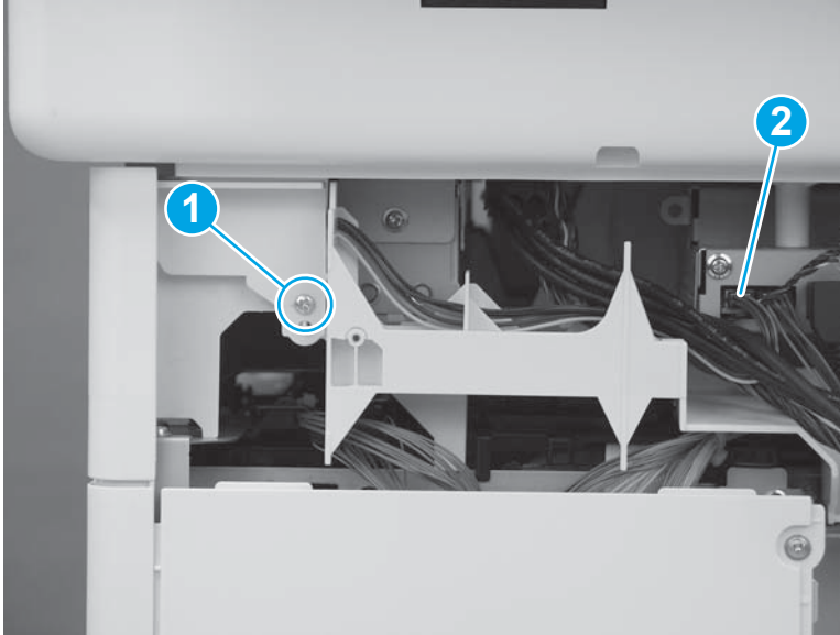
Figure 1-3299 Install one screw and connector
