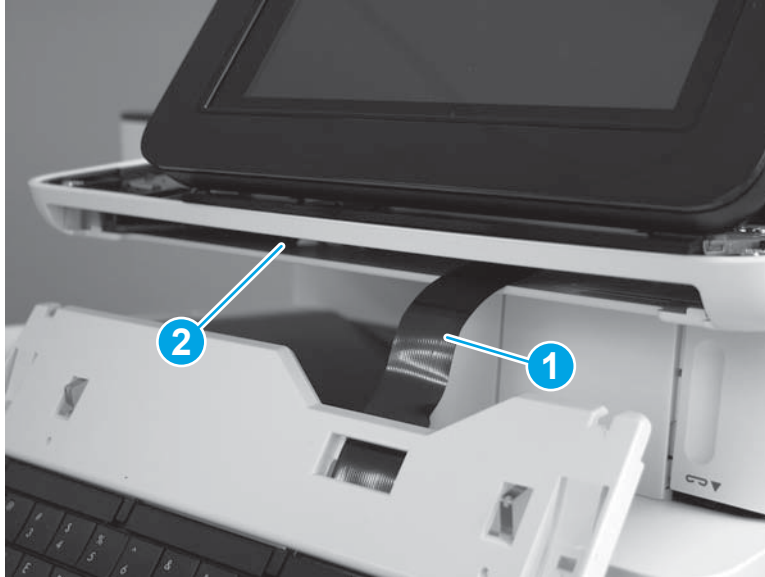
Figure 1-155 Install the flat cable through the slot
