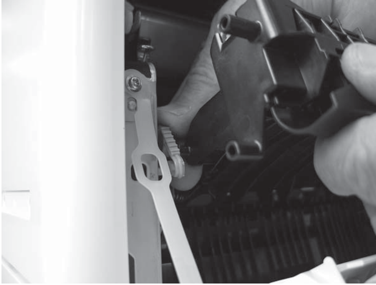
Figure 1-4284 Disengage the blue arm and pin
