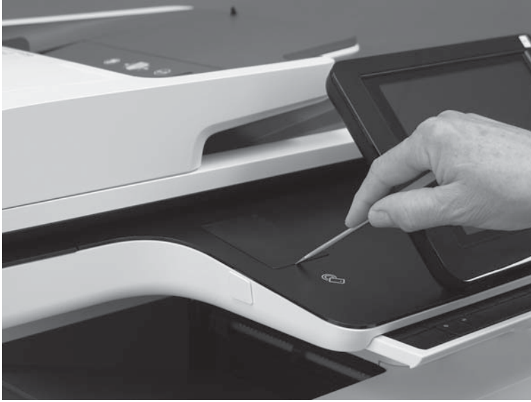
Figure 1-107 Release the HIP cover tabs
