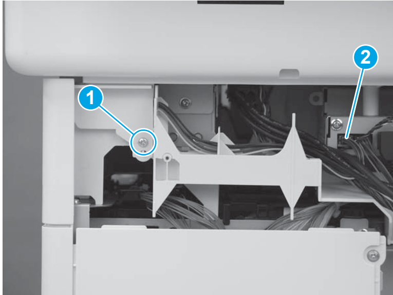
Figure 1-757 Remove one screw and connector
