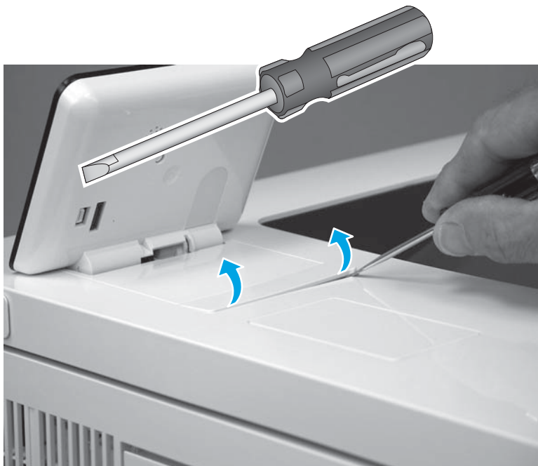
Figure 1-1006 Release the control-panel screws cover tabs
