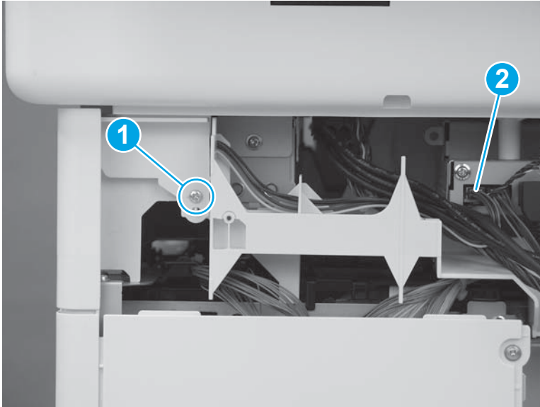
Figure 1-1110 Remove one screw and connector
