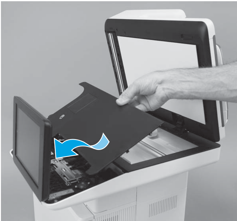
Figure 1-144 Position the control-panel cover on the printer
