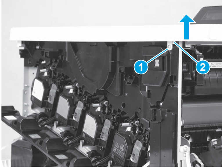
Figure 1-3663 Remove one screw and release one tab
