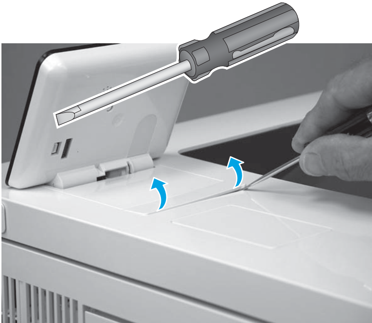
Figure 1-2325 Release the control-panel screws cover tabs
