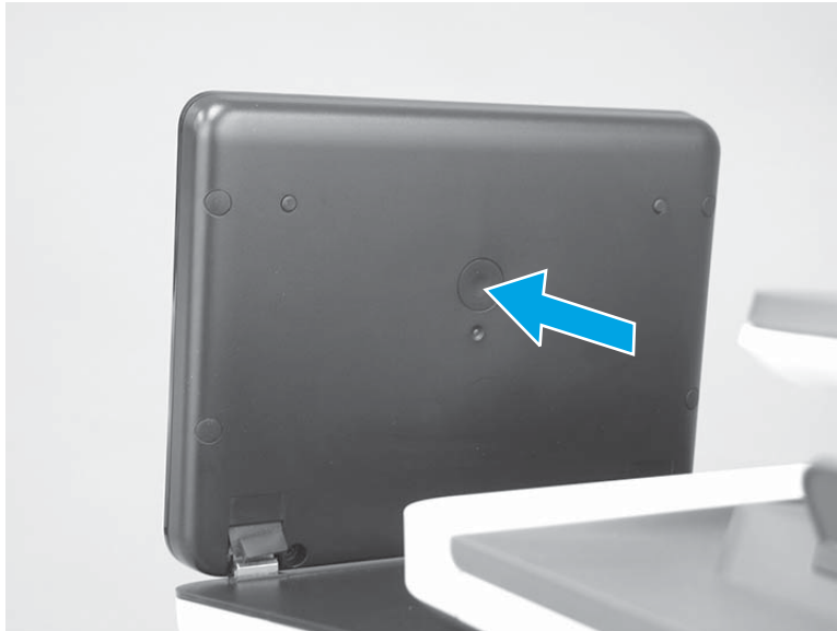
Figure 2-24 Press the diagnostics-access button
