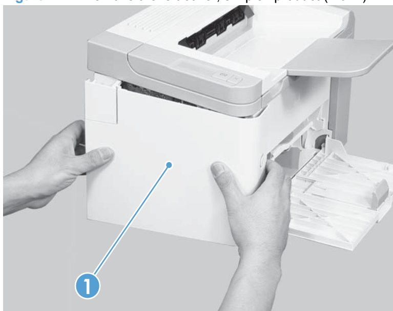
Figure 2-12 Remove the left cover, simplex product (4 of 4)
