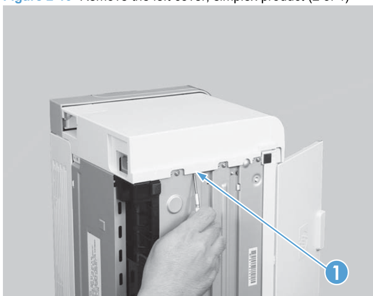
Figure 2-10 Remove the left cover, simplex product (2 of 4)
