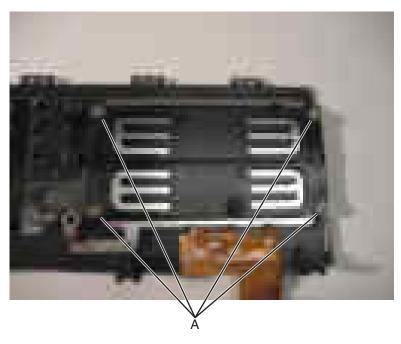
4 Remove the ground shield.
