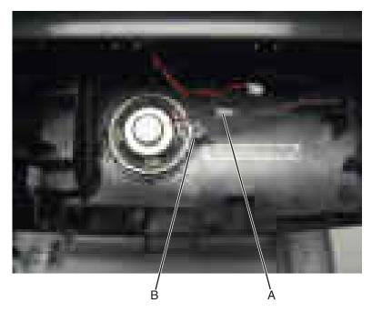
Slide the speaker off the scanner assembly.
