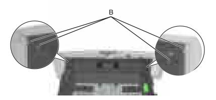
**4** Push out the top part of the drawer cover, and then remove the separator roll assembly.
