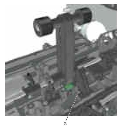
**17** Remove the ACM assembly with shaft.
