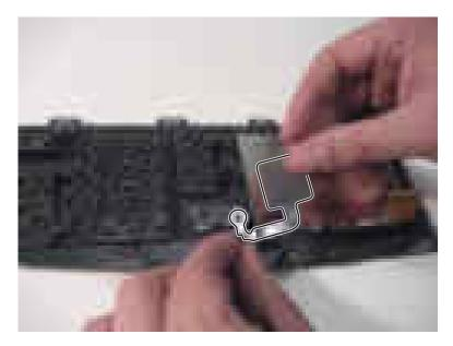
**5** Remove the light tube (B).
