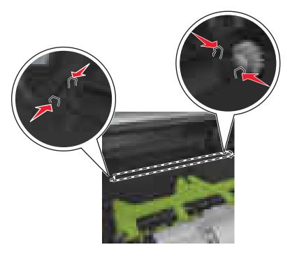
**2** Lift to remove the transfer roll.
