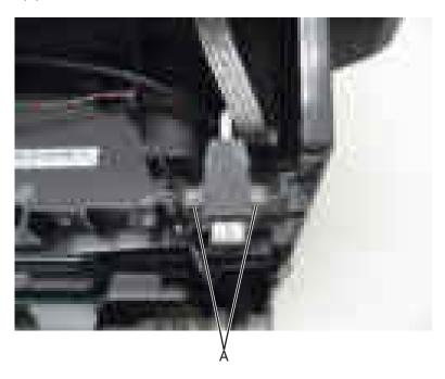
**3** Remove the USB cable bracket.
