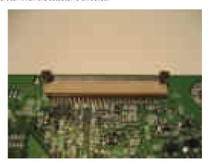
2 Insert the cable with the contacts on the cable facing up. Insert the cable on top of the actuator.
