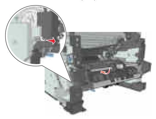
**10** Release the front guide from the guides at each end.
