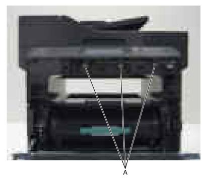
4 Lift the control panel assembly, disconnect the ribbon cable (JUICC1) from the UICC card, and then feed the ribbon cable through the wire channel.
