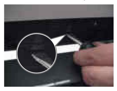
Disconnect the blade fastener (A) holding the ground cable to the ADF relay board.
