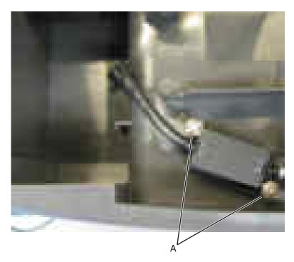
Feed the wireless cable through the channel on the left side of the printer.
