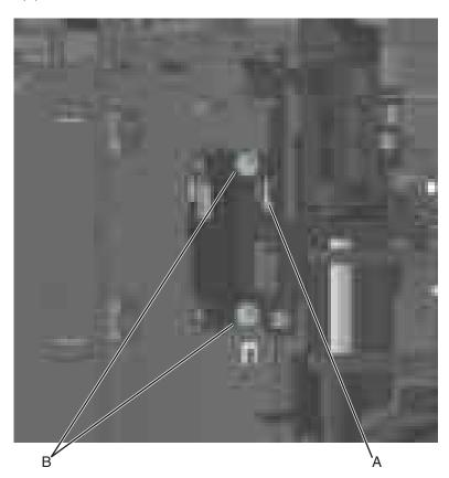
**9** Disconnect the cable from the sensor.
