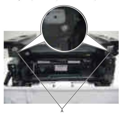
**3** Lift the top cover assembly, and remove.
