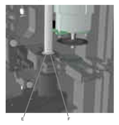
**13** Release the lock by sliding the bushing and then rotating it clockwise.
