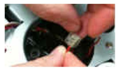
**f** Insert the red wire from the clutch into the IDC.
