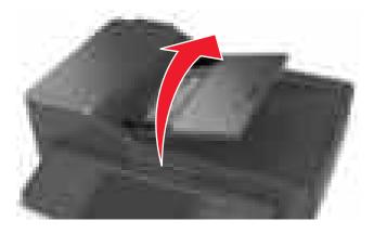
Hold the cushion by its handles, then peel it off the scanner.
