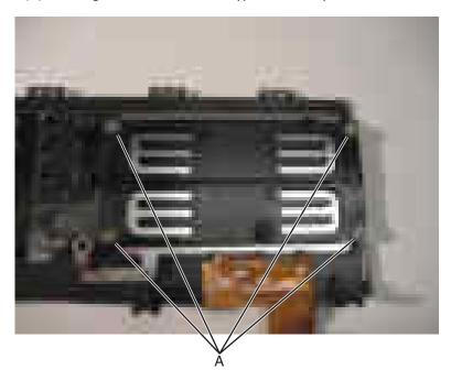
4 Remove the ground shield.
