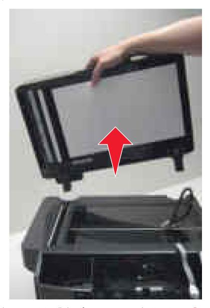
**Installation note:** After the new ADF is installed, perform scanner manual registration, see "Scanner manual registration" on page 178 and scanner calibration, see "Scanner calibration" on page 155.
