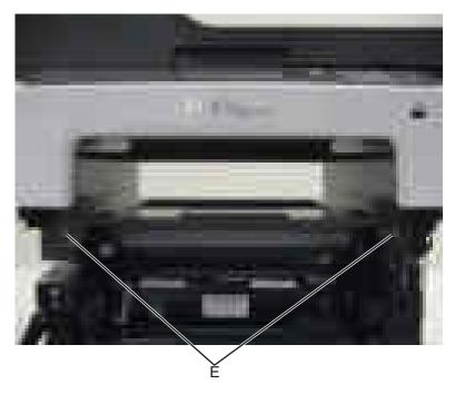
**12** Lift the scanner assembly, and remove.
