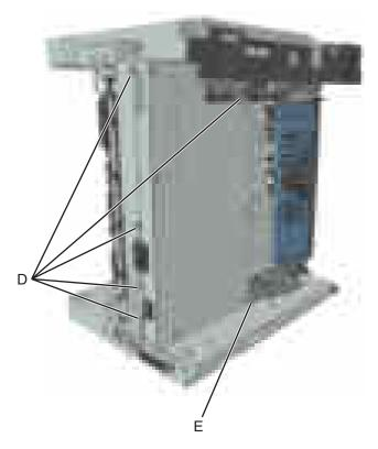
**7** Remove the power supply, and then disconnect the cable from the power supply.
