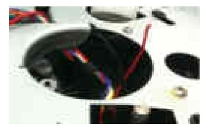
**b** On the replacement clutch, measure 4 inches from the clutch, and then cut the cable.
