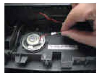
**9** Feed the speaker cable through the channel on the right side of the printer.
