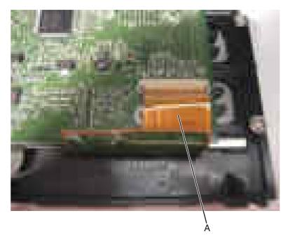
**3** Remove the five screws, and then remove the UICC.
