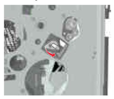
12 Pry the pointed end of the 2nd pickup pushing to release the locking pin underneath.
