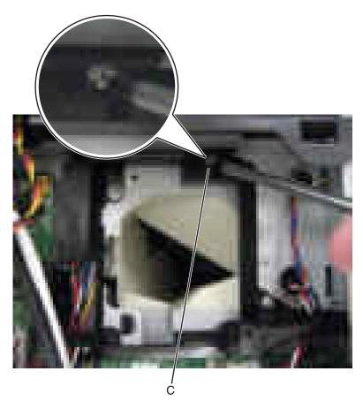
Remove the screw securing the rear left side of the scanner assembly to the printer frame.
