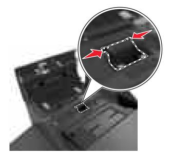
Pull away the separator roll and remove.
