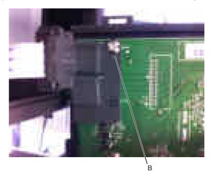
7 Disconnect the UICC cable from the controller card, and then remove the control panel assembly.
