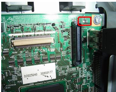
Figure 5: Fuse on the IPU
