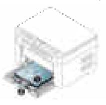
4. Pinch the paper length guide to adjust the guide so that it is flush up against the rear edge of the paper; then pinch the paper width guides so they are flush against the sides of the paper.
