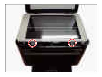
3. Lift up and release the scan glass.
