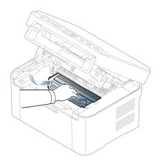
11. Close the inner cover and the scan unit in order. Printing automatically resumes.
