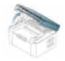
3. If the paper does not eject, remove the jammed paper by gently pulling it straight out.
