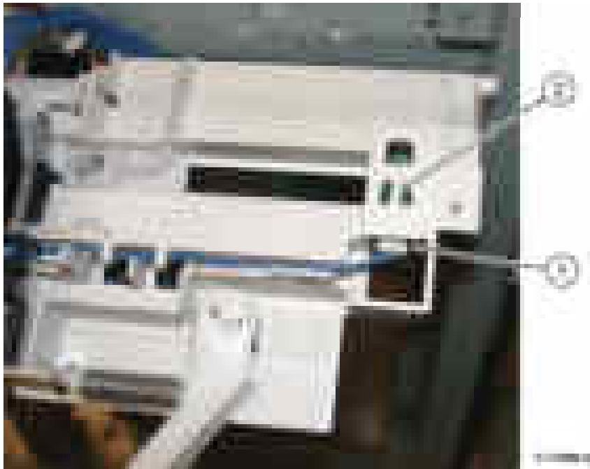
Figure 1 Tamper home sensor removal
